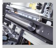
Continuous "V-Channel" for the efficient feeding of short bar sections.
