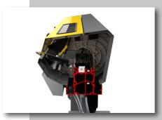
Torsion-resistant machine base made of extruded aluminium allows for optimal vibration dampening
