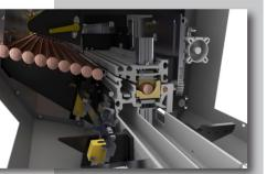
The movable guide segments automatically adapt to the required material bar diameters
